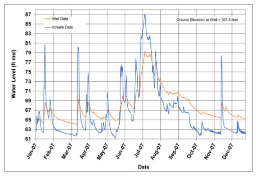
**Figure 3.** Comparison of measured water levels in the Colorado River and in the Colorado River Alluvium near the City of Wharton in 2007 (from URS and Baer Engineering 2007).
