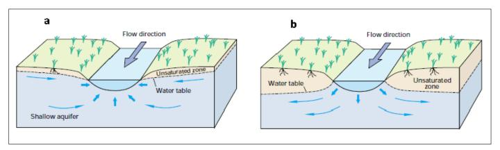
**Figure 1.** Schematic showing groundwater flow toward a gaining stream (a) and groundwater flow away from a losing stream (b) (modified from Winter et al. 1998).
