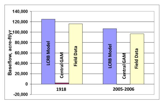
**Figure 4.** Comparison of measured baseflow along the Colorado River (Field Data) with simulated baseflow values from the LCRB groundwater model and from the Central Gulf Coast Groundwater Availability Model (data from Young et al. 2009; LCRB = Lower Colorado River Basin, GAM = groundwater availability model). The Field Data includes gain-loss studies performed with river gage data reported by Slade (2002) and Saunders (2006).
