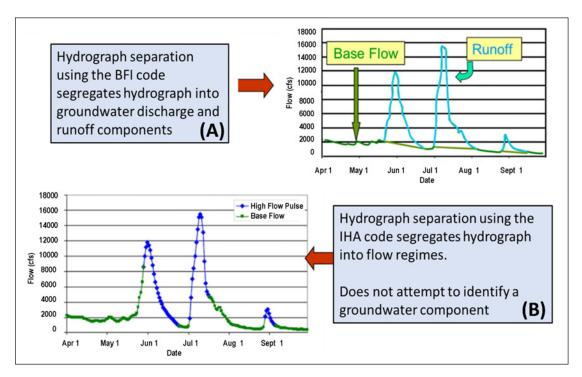
**Figure 5.** Analysis of a stream gage hydrograph by a surface water hydrologist using the IHA software (A) and by a groundwater hydrologist using the BFI software (B) (IHA = Indicators of Hydrologic Alteration; BFI = baseflow index).
